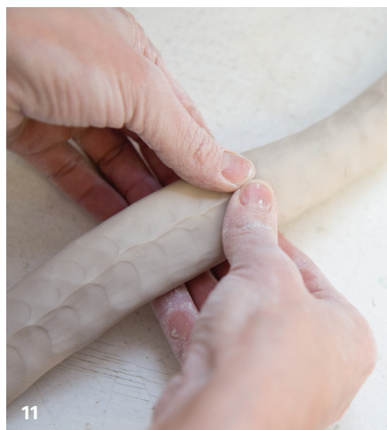
11 Create a handle by rolling out a coil to the appropriate diameter, then pinch up along the length to flatten and create a spine.
