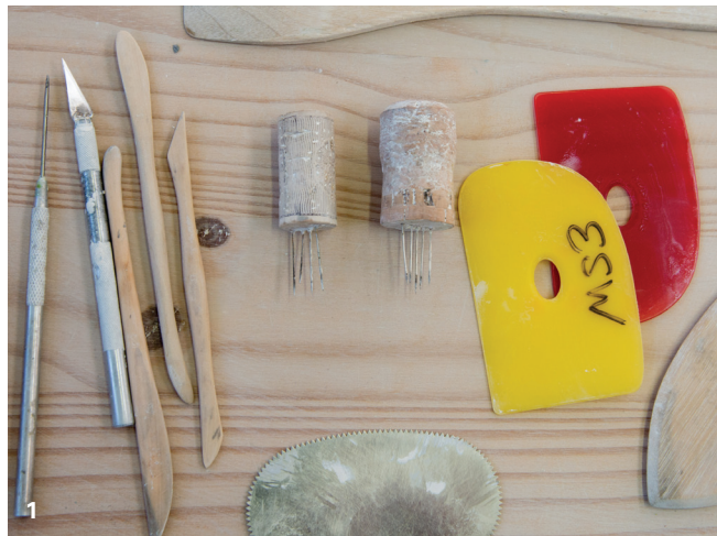
To build a pinch and coil pot, you'll need a few knife blades, a needle tool, wooden modeling tools, scoring tools, and ribs.
