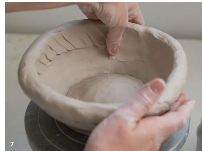
Level and score the surface, then place another coil on top. Join it to the pot using a criss-cross motion with your thumb.
